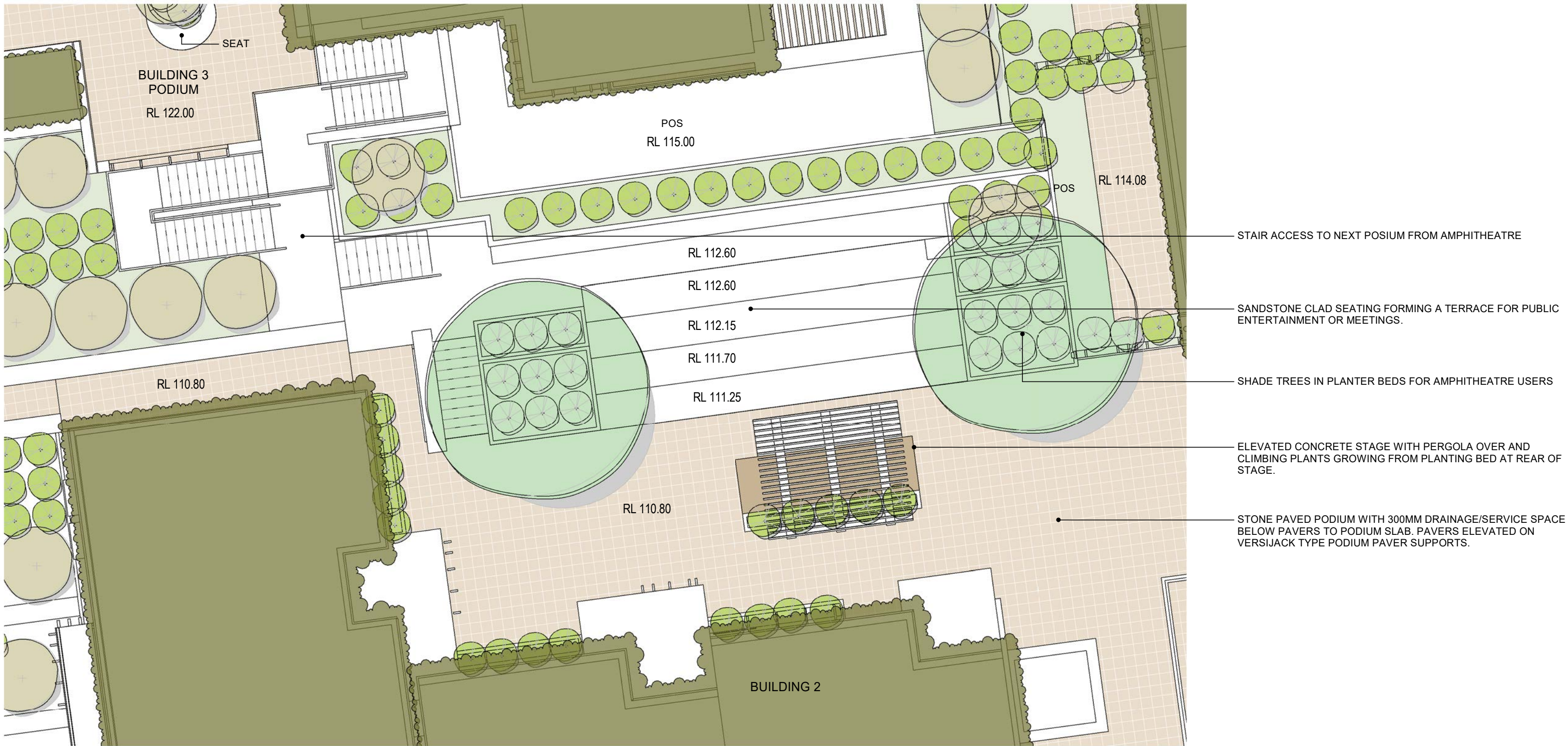
2 Central Communal Open Space Detail Plan 1 : 100
